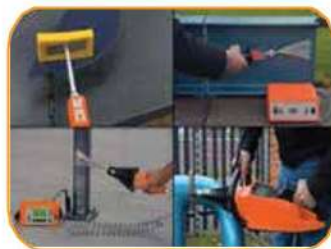
VACUUM BOX TESTING
