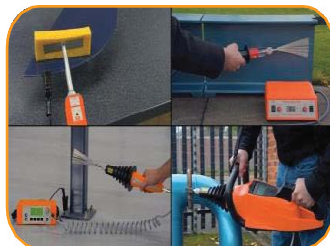
VACUUM BOX TESTING
